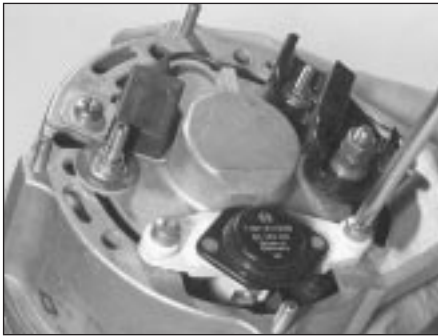
7.3a Undo the retaining screw and . . .
