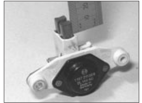
7.4 Measuring the brush lengths (Bosch alternator)
