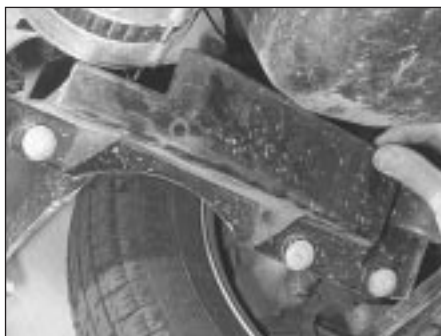
6.3 Removing the drivebelt splash guard (where fitted)
